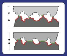
Above: Top section shows a low compression connection. Lower section shows the deformation of the plug and socket when compressed together. This compression displaces the soft tarnish as well as increasing the contact area.
